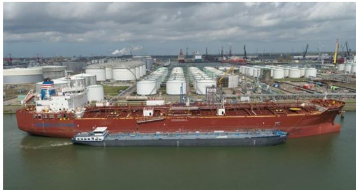
The tanker Takaroa Sun undergoing barge-to-ship methanol bunkering in Rotterdam
