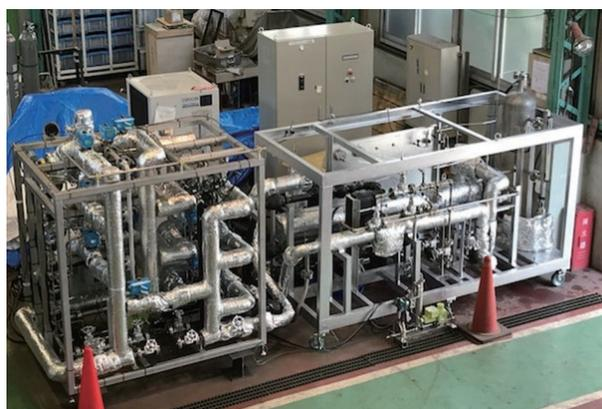
The compressor used in the demonstration testing
